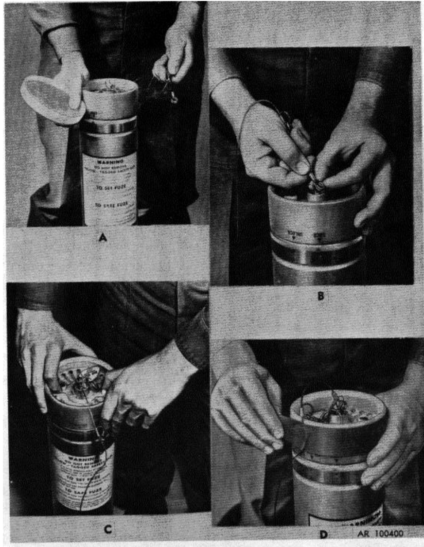
Figure 2-1. Attaching lanyard and setting fuze.
